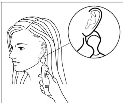
3. *Brush hair away if covering ear. Keeping the button depressed, lift probe from forehead, touch behind ear halfway down the mastoid process and slide down to the soft depression behind the earlobe.*
