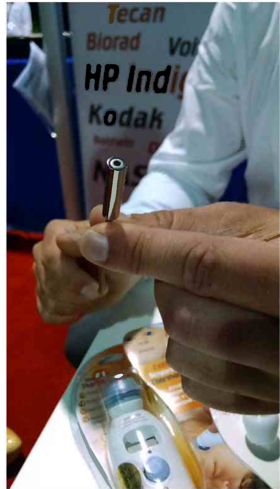
[Figure 1 | Exergen microIRt/c sensors contain are powerless, completely passive IR temperature sensors that come in a small package for a variety of industrial/embedded applications.]
